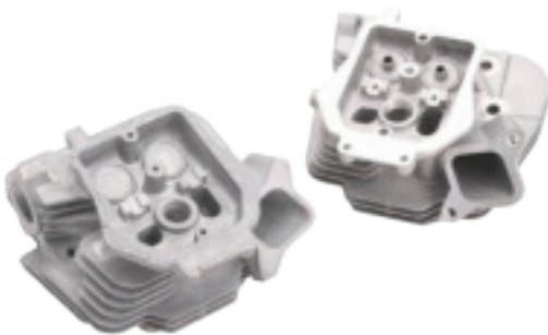
Figure 2.21 Engine Cylinder Head This die cast cylinder head required careful development and complex tooling to produce the configuration shown. Tooling and development costs were justified by the design improvements, high production rates, reduction of weight and reduced machining requirements provided by the die casting process.
