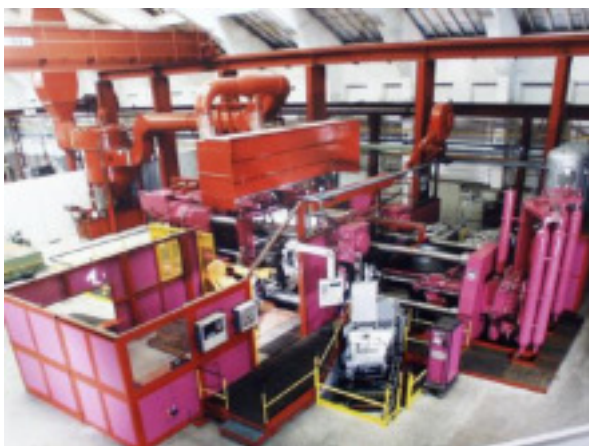
Figure 2.20 Automated Die Casting Cell The advanced equipment shown here has been used to create an automated die casting manufacturing cell. The sizable capital investment for this equipment is one of the processing costs associated with die castings.
